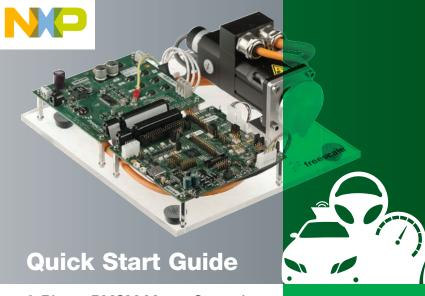
**3-Phase PMSM Motor Control Development Kit**with Qorivva MPC5643L MCU
