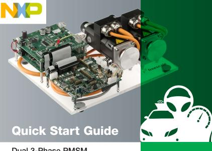
Dual 3-Phase PMSM Motor Control Development Kit with Qorivva MPC5643L MCU
