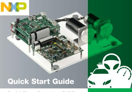
Dual 3-Phase Sensorless BLDC Motor Control Development Kit with Qorivva MPC5643L MCU
