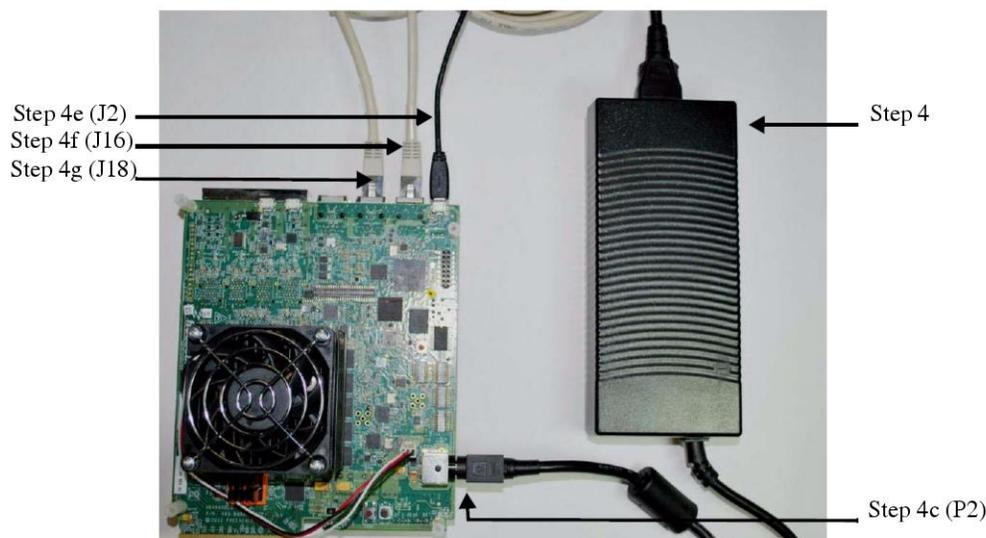
**Figure 2-2. Connecting the B4860 QDS Board**
