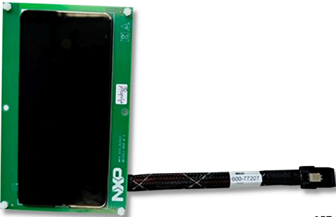
Figure 57. i.MX mini SAS cable with DSI-to-SDSB (Serialiser and Deserialiser) adapter
