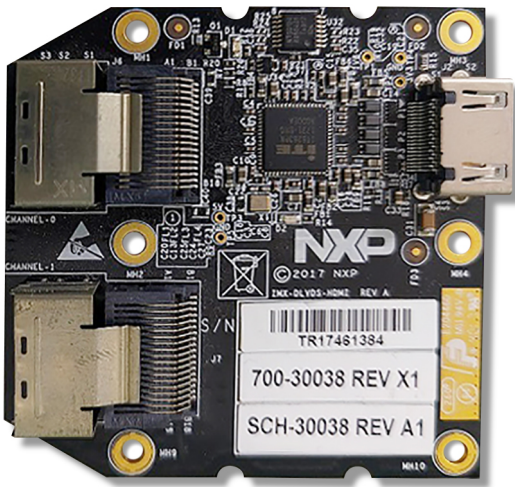
Figure 18. i.MX dual-channel LVDS-to-HDMI adapter
