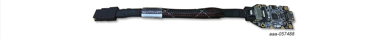
Figure 55. i.MX mini SAS cable with LVDS-to-HDMI adapter
