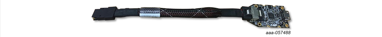
Figure 39. i.MX mini SAS cable with LVDS-to-HDMI adapter
