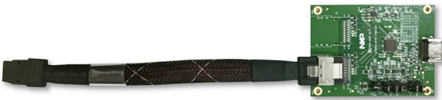
Figure 56. i.MX mini SAS cable with DSI-to-HDMI4K adapter
