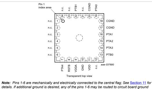
plane, or the central flag may be connected to circuit board ground plane with vias.
