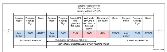
Figure 14. Sequence of events when NBPx notifies the external host of an event and the external host clears the SPIOPS register
