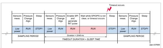
Figure 15. Sequence of events when NBPx notifies the external host of an event but the external host does not clear the SPIOPS register
