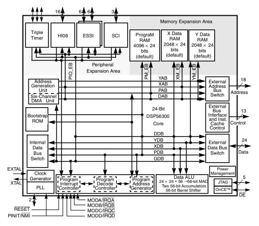
The DSP56303 is intended for use in telecommunication applications, such as multiline voice/data/ fax processing, video conferencing, audio applications, control, and general digital signal processing.
