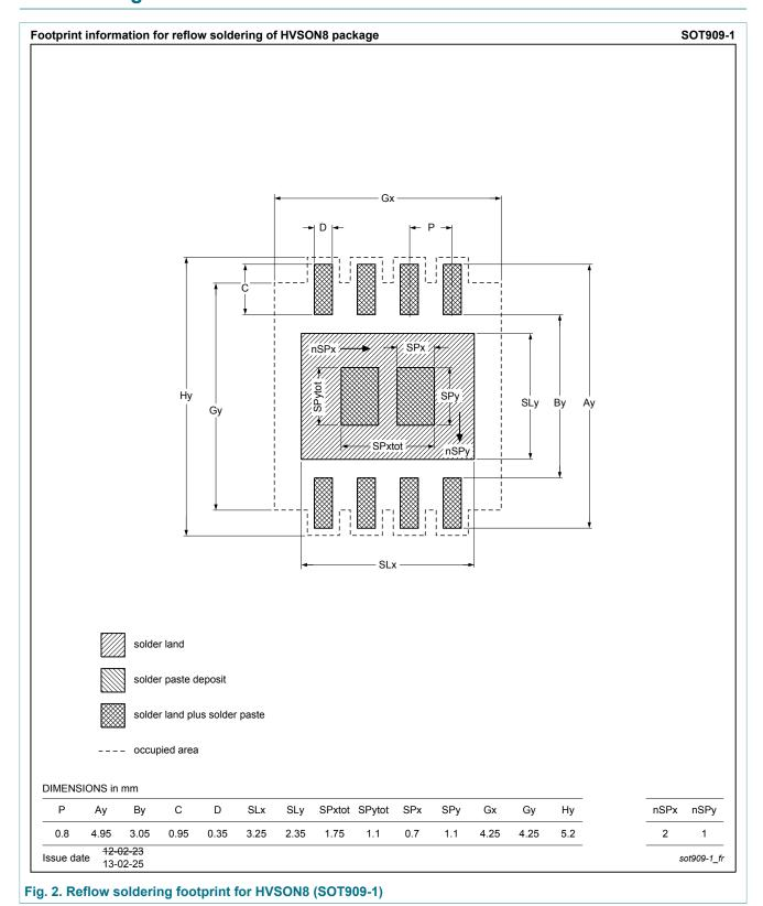
plastic thermal enhanced very thin small outline package; no leads; 8 terminals; body 4 x 4 x 0.85 mm
