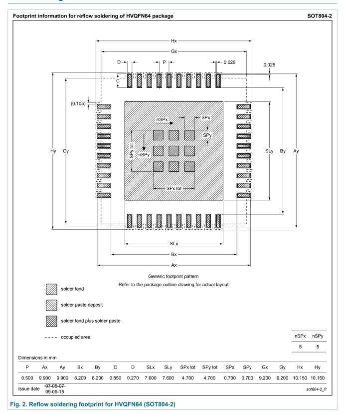
plastic thermal enhanced very thin quad flat package; no leads; 64 terminals; body 9 x 9 x 0.85 mm
