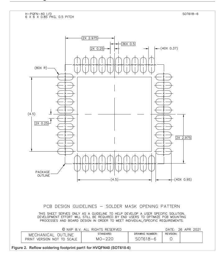
HVQFN40, plastic thermal enhanced very thin quad flat package; no leads; 40 terminals; 0.5 mm pitch, 6 mm x 6 mm x 0.85 mm body
