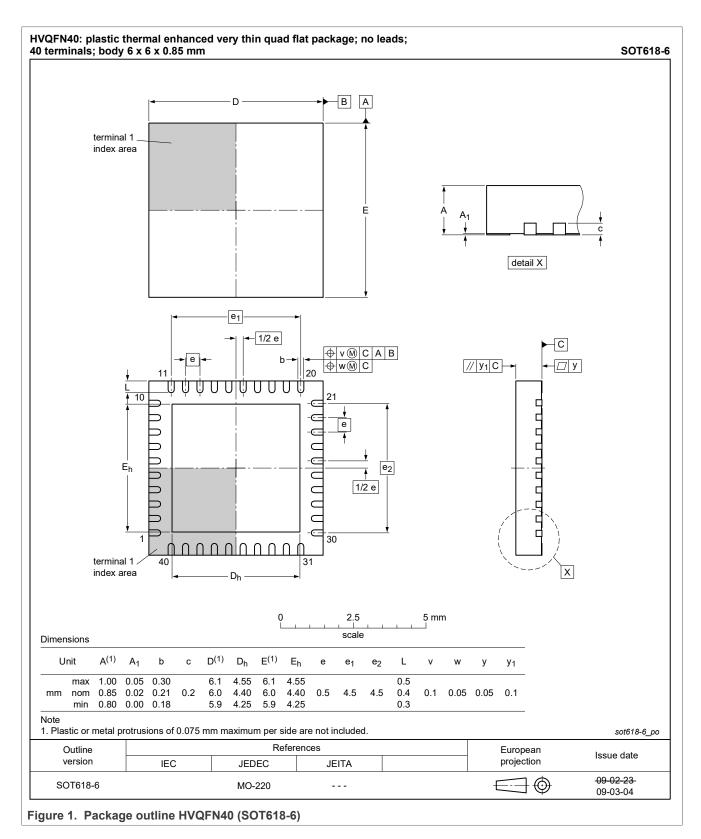
HVQFN40, plastic thermal enhanced very thin quad flat package; no leads; 40 terminals; 0.5 mm pitch, 6 mm x 6 mm x 0.85 mm body
