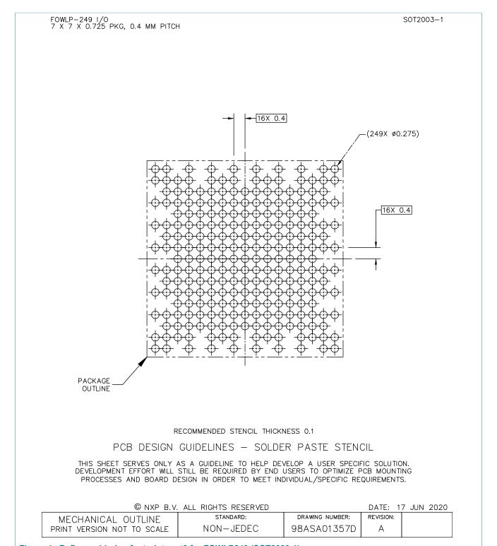
Figure 4. Reflow soldering footprint part3 for FOWLP249 (SOT2003-1)
