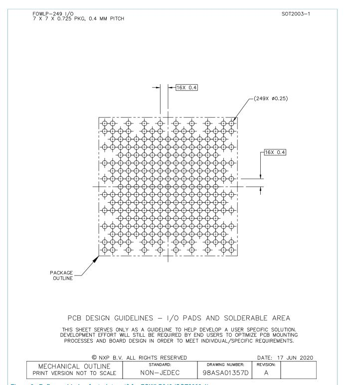
Figure 3. Reflow soldering footprint part2 for FOWLP249 (SOT2003-1)
