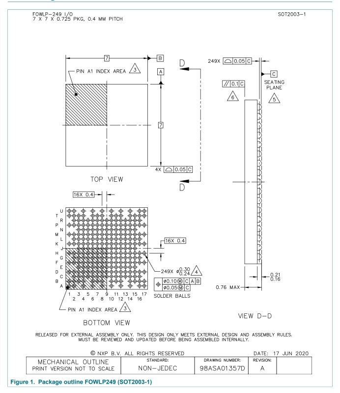
FOWLP249, fan-out wafer-level package, 249 terminals, 0.4 mm pitch, 7 mm x 7 mm x 0.725 mm body
