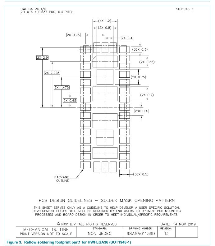
HWFLGA36, plastic thermal enhanced very very thin fine-pitch land grid array package, 0.4 mm pitch, 2.1 mm x 6 mm x 0.637 mm body
