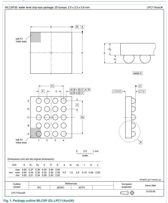
wafer level chip-size package; 20 bumps
