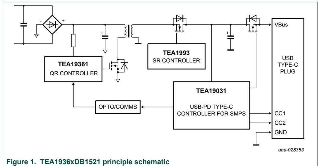
Figure 1. TEA1936xDB1521 principle schematic
