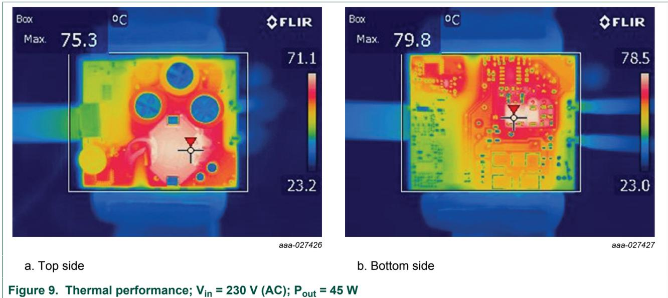
**Note:** Typical temperature distribution at  $T_{amb} = 25\text{ °C}$ ; PCB in free air, natural convection, and radiation only. For the TEA1936xDB1521 demo board, the voltage levels must not exceed 20 V also. Current limit levels must not exceed 3 A. Power limit levels must not exceed 45 W.
