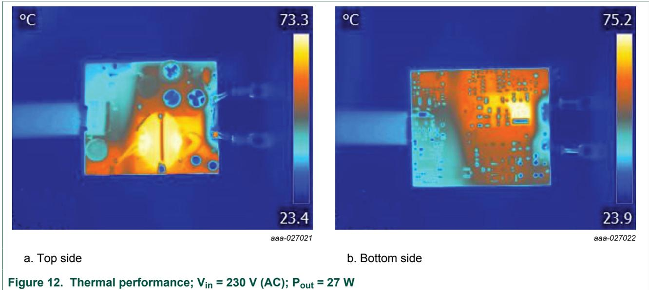
**Note:** Typical temperature distribution at  $T_{amb} = 25 \text{ °C}$ ; PCB in free air, natural convection, and radiation only.
