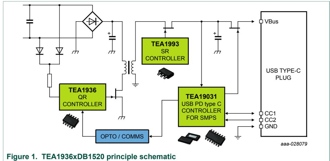
Figure 1. TEA1936xDB1520 principle schematic
