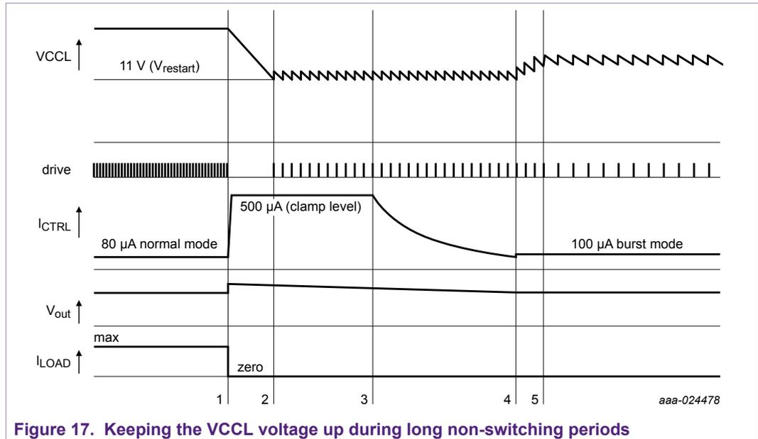
Figure 17. Keeping the VCCL voltage up during long non-switching periods
