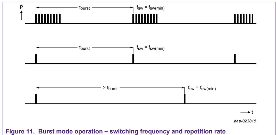
Figure 11. Burst mode operation – switching frequency and repetition rate
