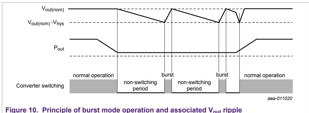
Figure 10. Principle of burst mode operation and associated  $V_{out}$  ripple
