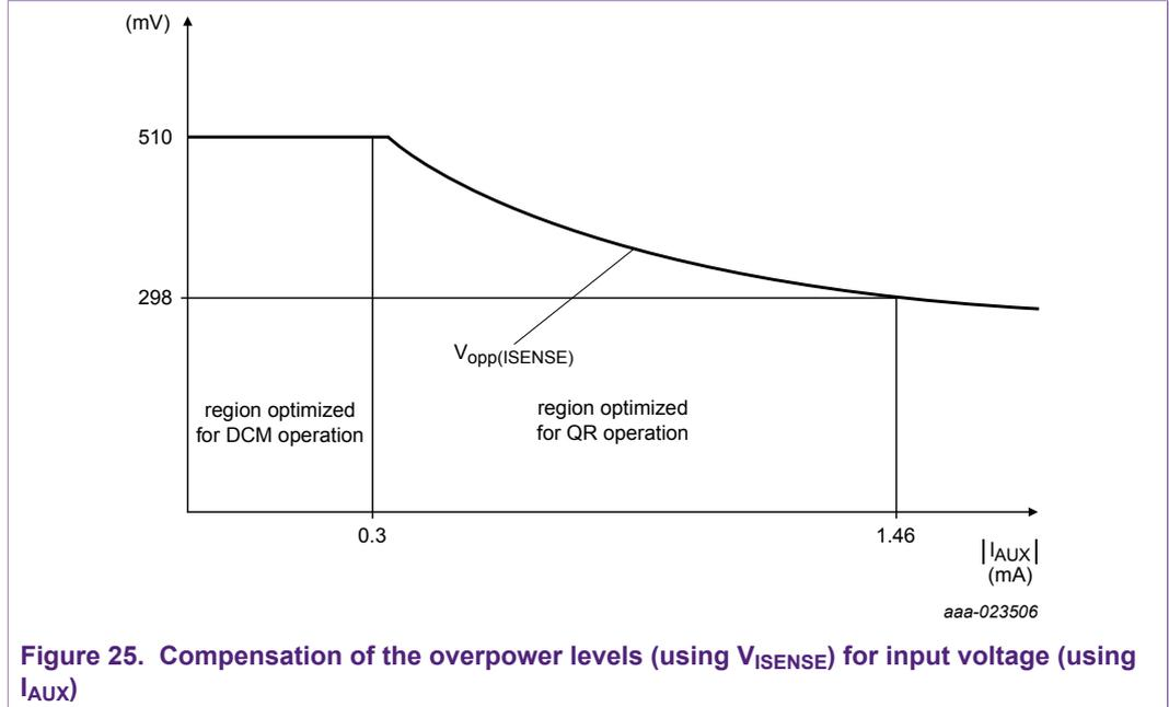
Figure 25. Compensation of the overpower levels (using  $V_{I\text{SENSE}}$ ) for input voltage (using  $I_{\text{AUX}}$ )
