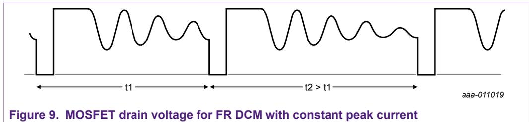
Figure 9. MOSFET drain voltage for FR DCM with constant peak current
