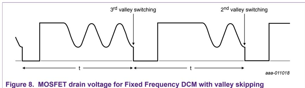
Figure 8. MOSFET drain voltage for Fixed Frequency DCM with valley skipping
