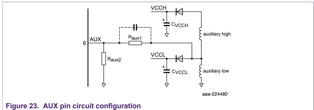
Figure 23. AUX pin circuit configuration
