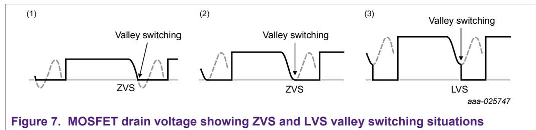
Figure 7. MOSFET drain voltage showing ZVS and LVS valley switching situations
