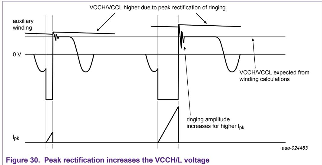
Figure 30. Peak rectification increases the VCCH/L voltage
