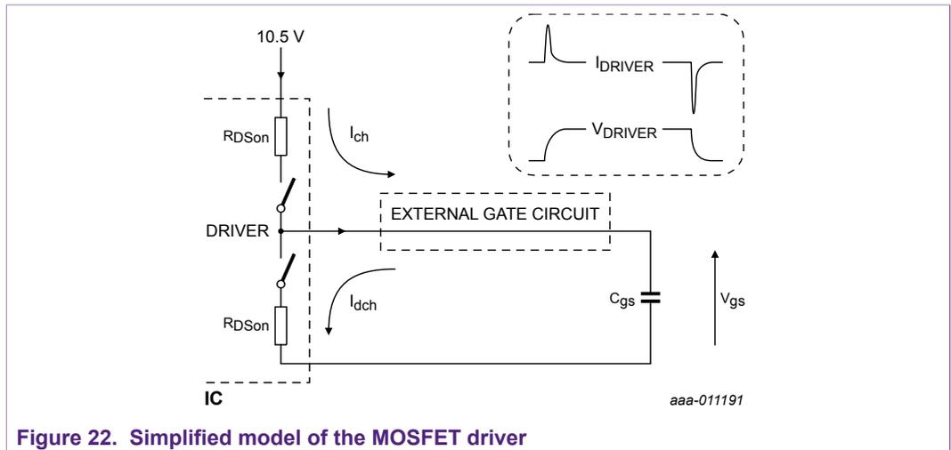
Figure 22. Simplified model of the MOSFET driver
