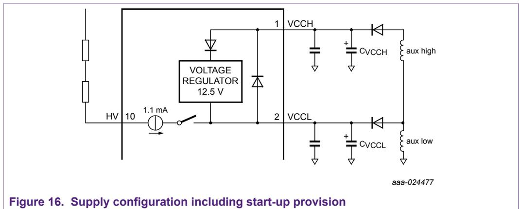
Figure 16. Supply configuration including start-up provision
