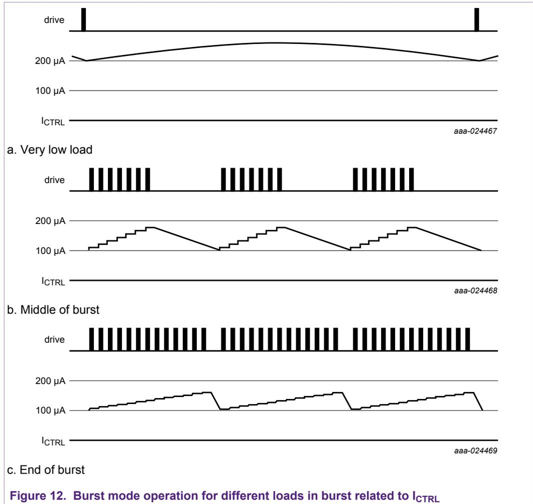
At very low loads, only one switching cycle is required to make  $I_{CTRL}$  increase to exceed 100  $\mu\text{A}$ . Only when the  $I_{CTRL}$  drops again to below 100  $\mu\text{A}$ , the next stroke is made. Depending on the winding ratio of the transformer and the output voltage, it is possible that two or three strokes are required. Except for the number of strokes per burst cycle, the behavior remains the same.
