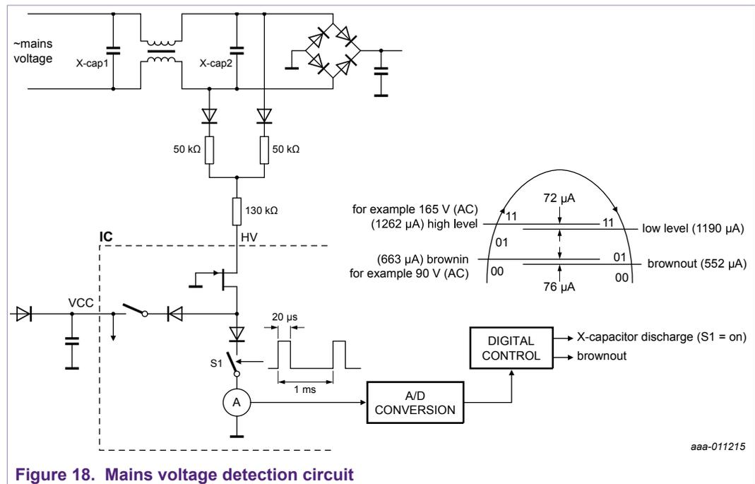
Figure 18. Mains voltage detection circuit
