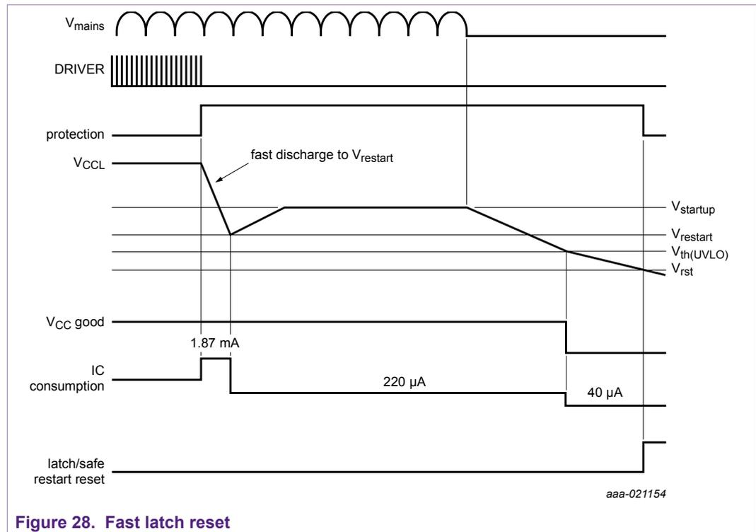
**Figure 28. Fast latch reset**
