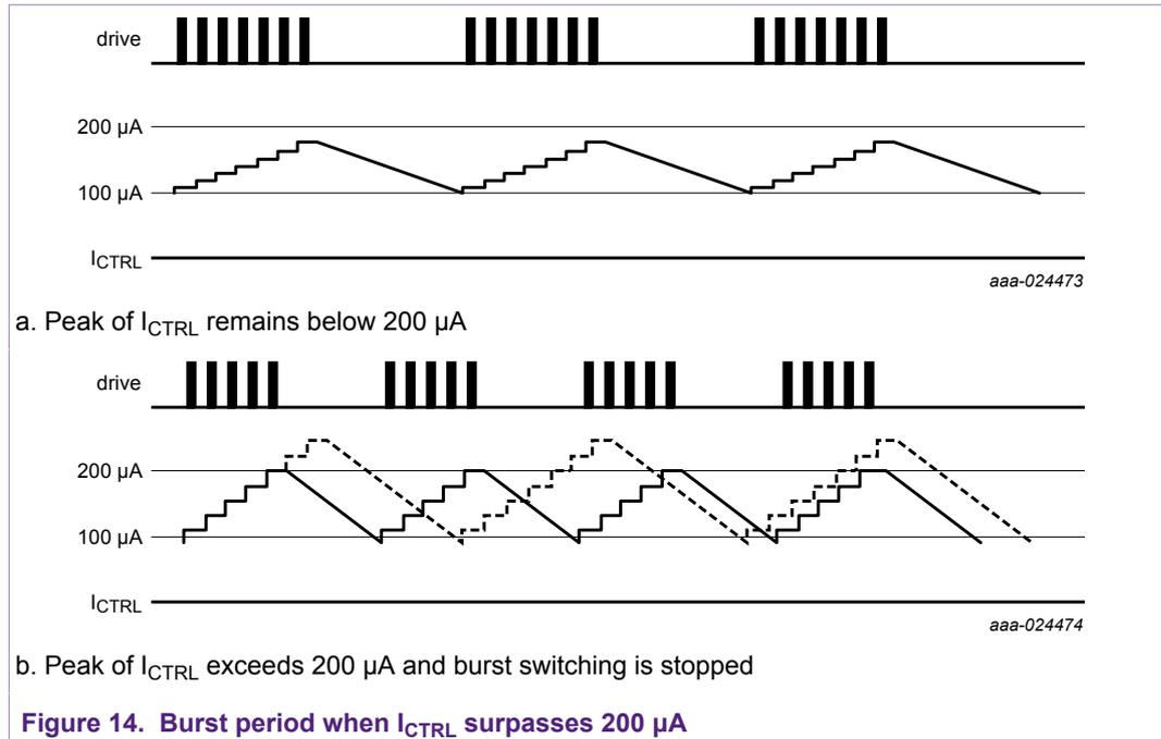
Figure 14(b) shows that the burst period reduces when  $I_{CTRL}$  exceeds the 200  $\mu A$  level. The dashed  $I_{CTRL}$  line indicates the intended (precalculated) behavior.
