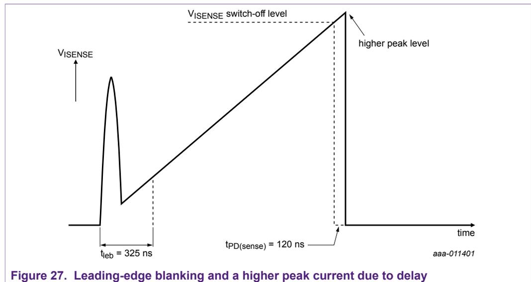
Under extreme conditions, di/dt can also rapidly increase because the transformer starts to saturate. The di/dt slope depends on the transformer and converter design. These saturation conditions must be avoided because the converter operation is unpredictable.
