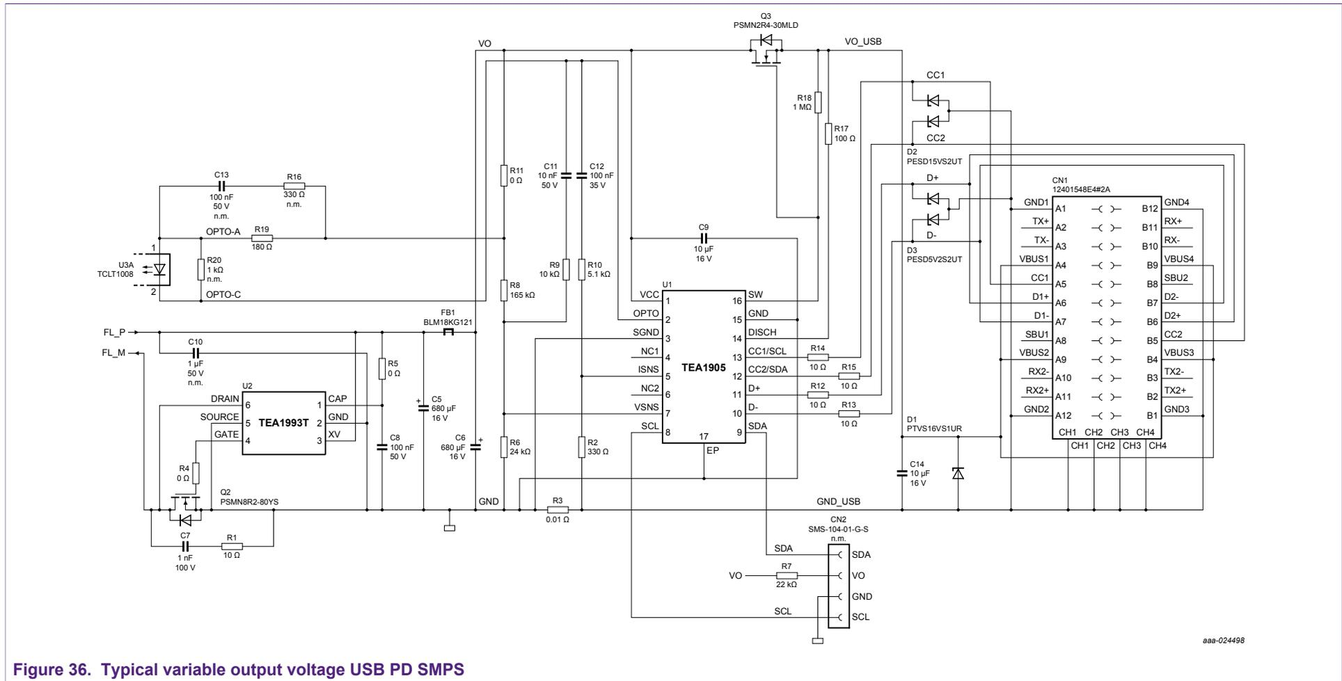
Figure 36. Typical variable output voltage USB PD SMPS
