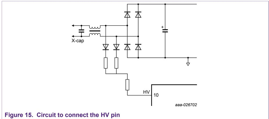
Figure 15. Circuit to connect the HV pin
