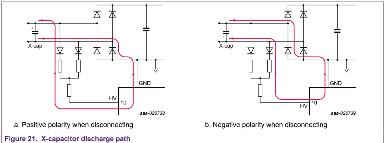
Figure 21. X-capacitor discharge path
