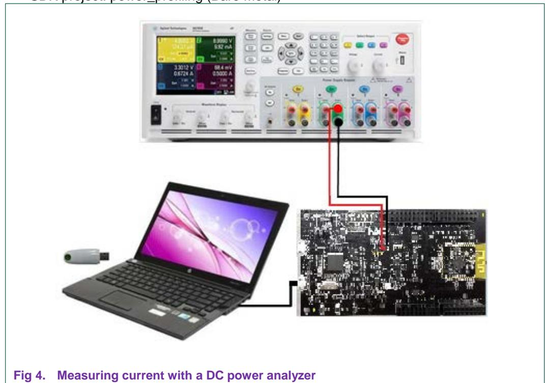
Fig 4. Measuring current with a DC power analyzer
