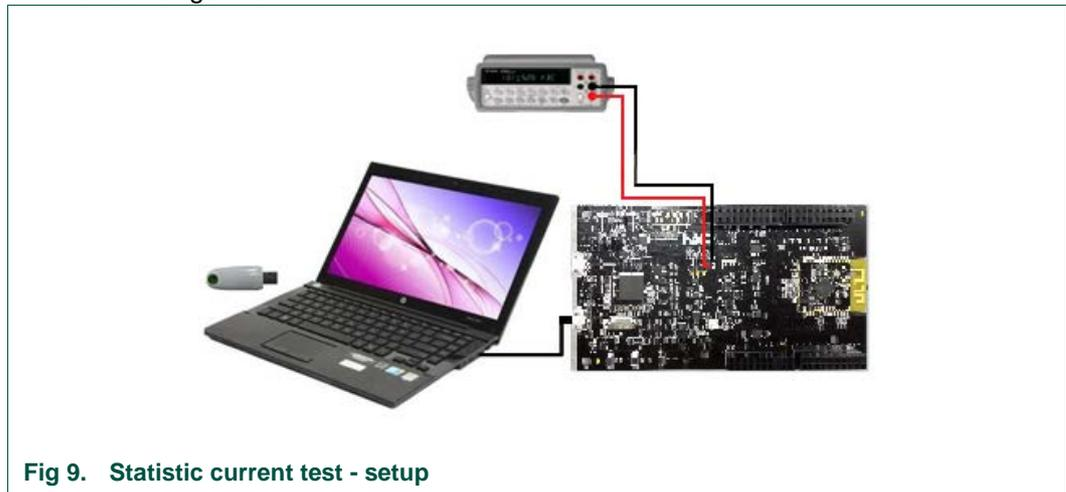
**Fig 9. Statistic current test - setup**
