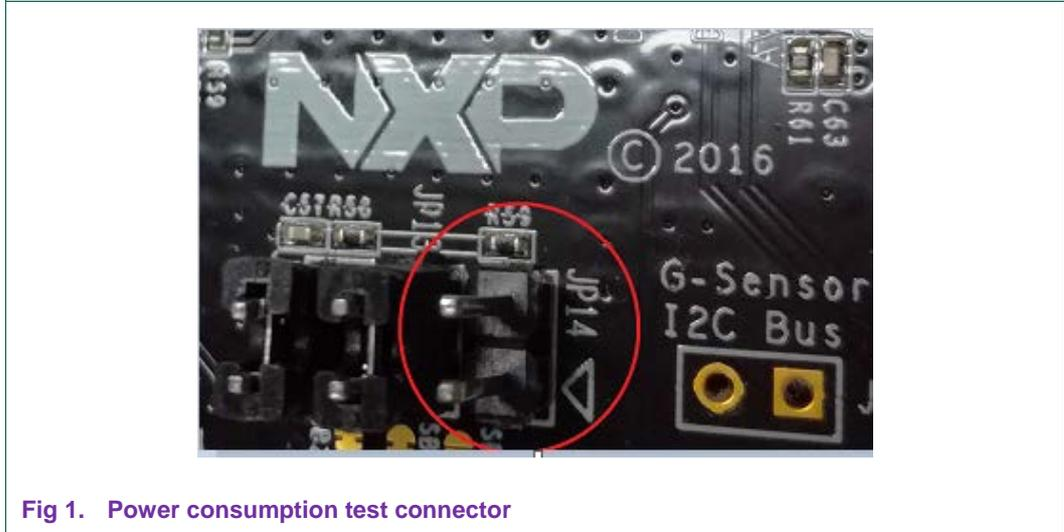
Fig 1. Power consumption test connector
