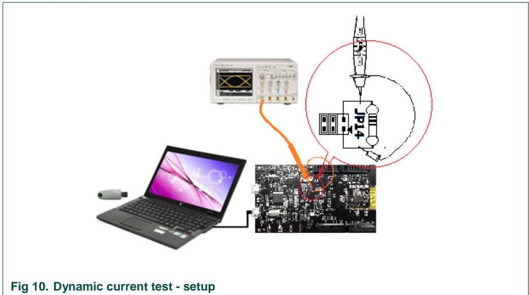
Fig 10. Dynamic current test - setup
