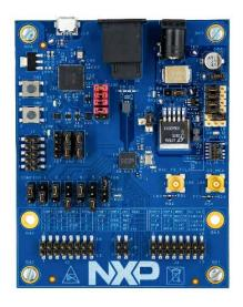
The TJA1103EVB evaluation board is a low-cost hardware development tool that supports the functional evaluation of the 100BASE-T1 Ethernet PHY TJA1103. To flexibly adapt to different application use cases, all configuration options can be selected via jumpers and all logic interfaces can be accessed via pin headers.
