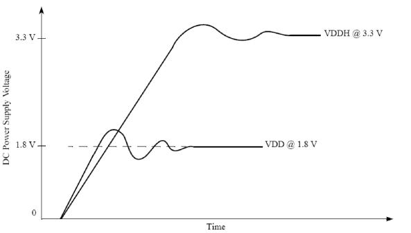
Figure 1. Power Supply Ramping
