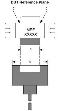
Figure 2. Illustration of the Instantaneous Impedance Change and Need for MSTEP Blocks
