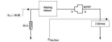
Figure 6. Generalized Schematic Used to Optimize Matching Network
