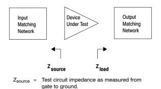
Z<sub>load</sub> = Test circuit impedance as measured from drain to ground.
