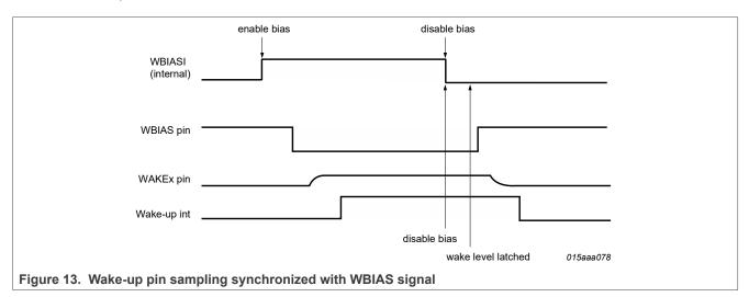
The sampling of the wake-up pins can be synchronized with the WBIAS signal by setting bits WSE1 and WSE2 in the Int\_Control register to 1 (if WSEx = 0, wake-up pins are sampled continuously). The sampling will be performed on the rising edge of WBIAS (see Figure 13). The sampling time, 16 ms or 64 ms, is selected via the Wake Bias Control bit (WBC) in the Mode\_Control register.
