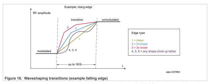
The shaping related register settings are stored in a lookup table located in EEPROM, and selected dependent on the actual detected detuning condition.
