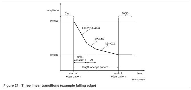
The transition patterns are used as implicit pre-distortion to compensate effects of TX loading circuitry (for example, resonant circuitry parameters) to the emitted RF envelope.
