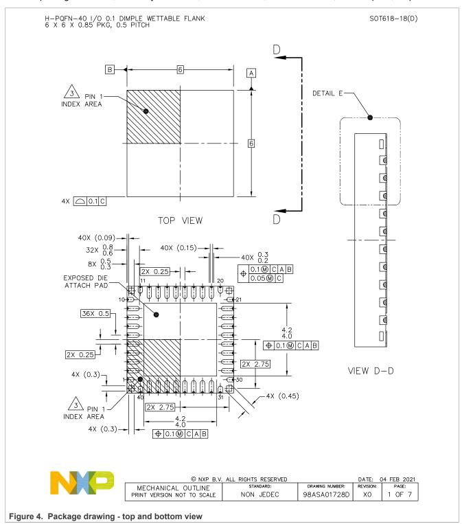
H-PQFN-40 I/O 0.1 DIMPLE WETTABLE FLANK 6 X 6 X 0.85 PKG, 0.5 PITCH SOT618-18(D) (0.2)-0.08 C (0.1) 0.05(0.3) -(0.25) 2X (0.05) С SEATING PLANE -(0.15) (0.5)DETAIL E VIEW ROTATED 90' CW © NXP B.V. ALL RIGHTS RESERVED DATE: 04 FEB 2021 MECHANICAL OUTLINE PRINT VERSION NOT TO SCALE DRAWING NUMBER: STANDARD: PAGE: NON JEDEC 98ASA01728D X0 2
