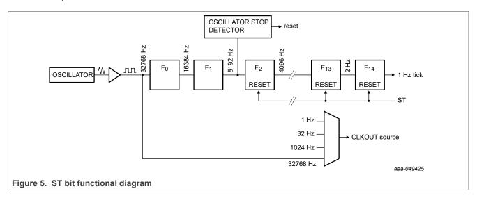
The ST bit function will not affect the output of 32.768 kHz on CLKOUT, but will stop the generation of 1.024 kHz, 32 Hz, and 1 Hz.
