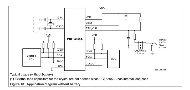
Bootable CPU RTC with two I<sup>2</sup>C buses, 128 byte SRAM and alarm function
