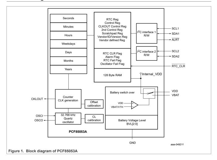
Bootable CPU RTC with two I<sup>2</sup>C buses, 128 byte SRAM and alarm function
