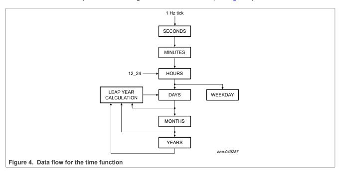
During read operations, the time registers are copied into an output register. The RTC continues counting in the background. When reading or writing the time it is very important to make a read or write access in one go, that is, setting or reading seconds through to years should be made in one single access. Failing to comply with this method could result in the time becoming corrupted.
