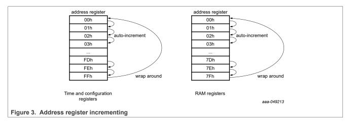
All registers are designed as addressable 8-bit parallel registers although not all bits are implemented.
