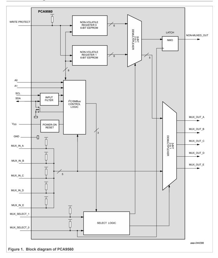
Dual 5-bit multiplexed 1-bit latched I<sup>2</sup>C-bus EEPROM DIP switch
