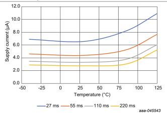
Figure 25. Supply current versus conversion time and temperature ( $V_{CC} = 1.8 \text{ V}$ , bus inactive)
