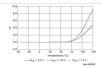
Figure 24. Shutdown current versus temperature
