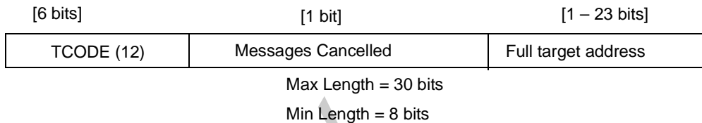
Figure 20-25. Indirect Branch Synchronization Message Format (PTSM = 0)
