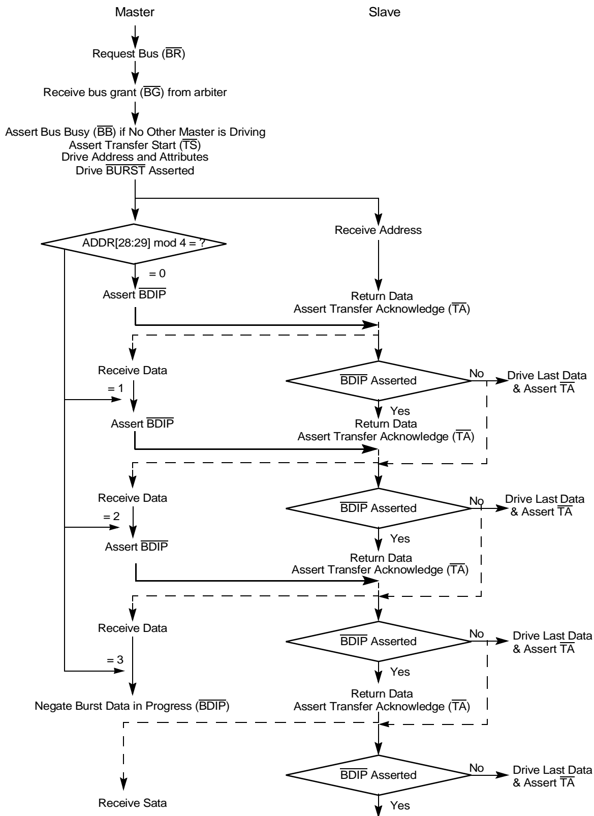
Figure 9-11 Basic Flow Diagram Of A Burst Read Cycle
