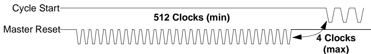
Figure 10-5 Master Reset Configuration Timing
