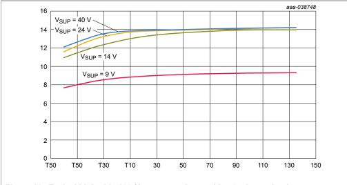
Figure 10. Typical high-side 100 % on gate voltage with 5.0 μA gate load
