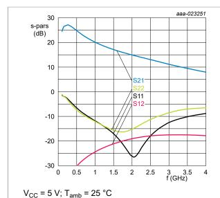
Figure 19. Wideband S-parameters as function of frequency Gain mode; typical values
