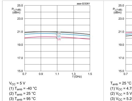
Figure 27. Output power at 1 dB gain compression as a function of frequency Gain mode; typical values
