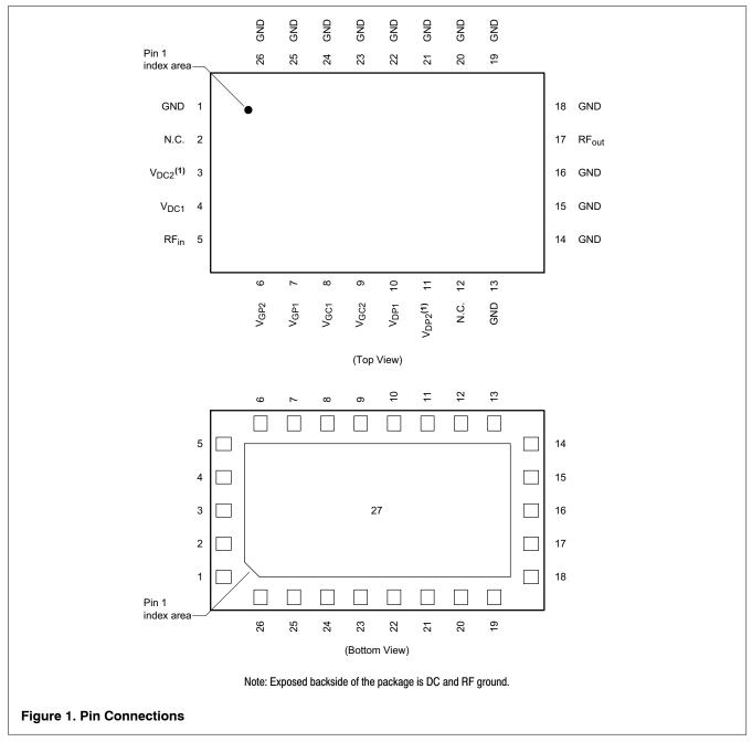
1.  $V_{DC2}$  and  $V_{DP2}$  are DC coupled internal to the package and must be powered by a single DC power supply.
