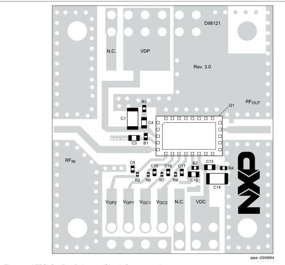
Figure 2. AFSC5G26E38 Reference Circuit Component Layout
