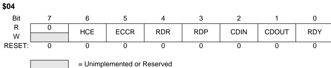
Figure 3-5 Smartmedia Interrupt Status Register(SMISR)
