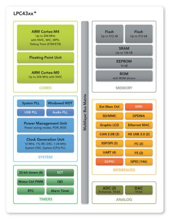
\*The LPC4370 adds an 80Msps 12-bit ADC and a subsystem with a second Cortex-M0 peripheral handler.
