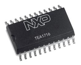
NXP resonant power supply controller TEA1716 with integrated PFC
