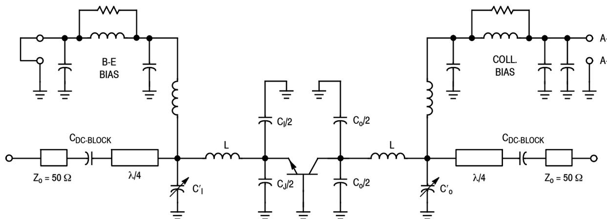
Figure 1. Schematic Representation of Test Fixture
