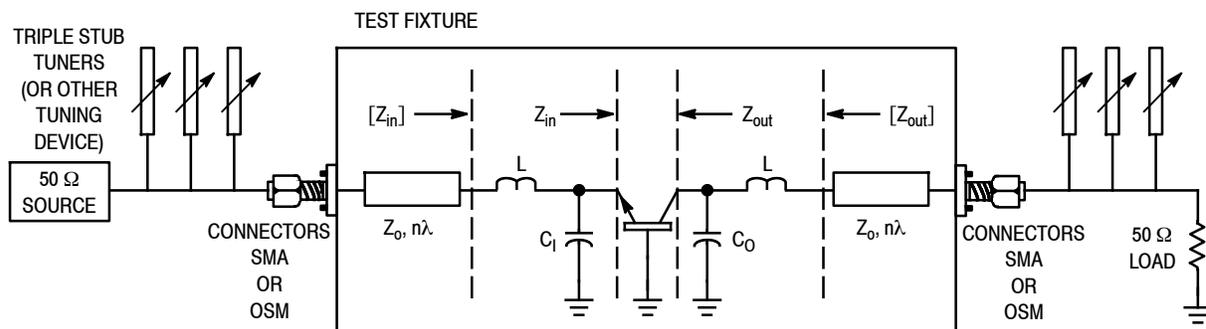
**Figure 5. Basic Circuit to Measure  $Z_{in}$ ,  $Z_{out}$**
