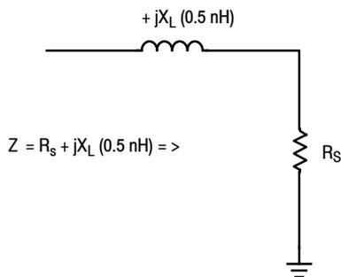
**Figure 2. Equivalent Circuit for  $Z_{in}$  or  $Z_{out}$**
