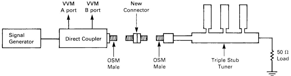
**Figure 8. Test Setup to Measure Stub Tuner w/Load**
