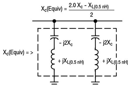
**Figure 4. Equivalent Reactance for Capacitors in Parallel**
