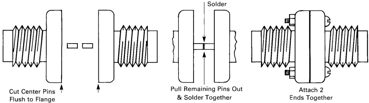
**Figure 7. Maintaining Reference Plane**
