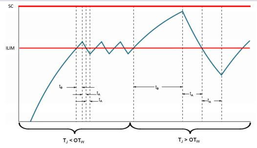
Figure 1. Active current limiting with synchronous rectification and thermal management
