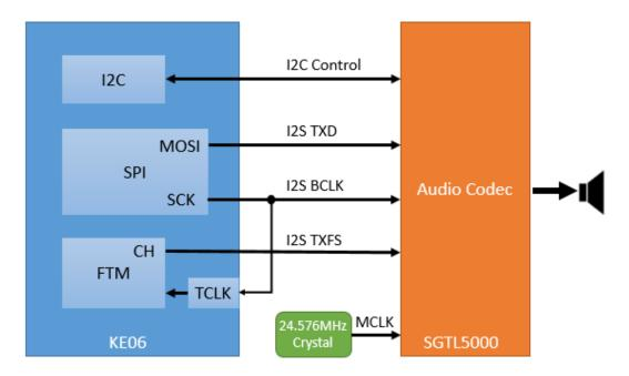
Figure 1. System Diagram
