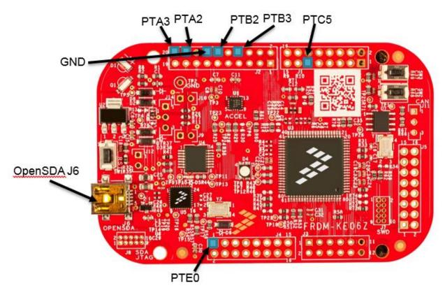
Figure 4. FRDM-KE06Z and Used Pins
