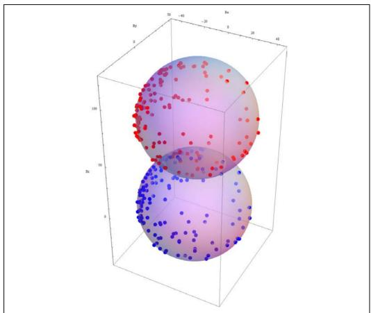
Fig 1. Uncalibrated (red) and calibrated (blue) measurements from a simple hard iron environment
