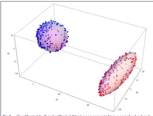
Fig 2. Uncalibrated (red) and calibrated (blue) measurements from a complex hard and soft iron environment
