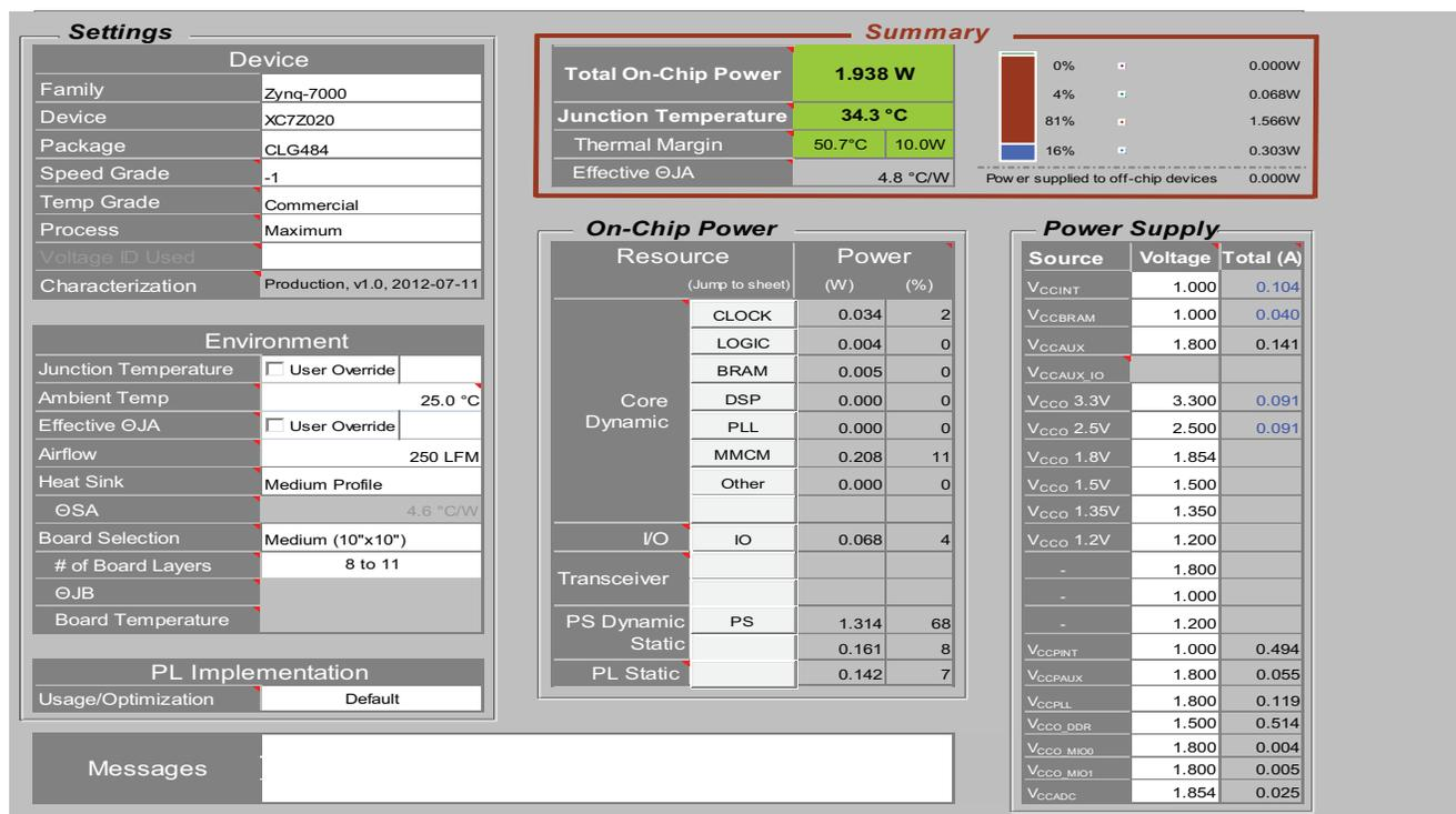
Figure 4. Power estimation data for use case 1
