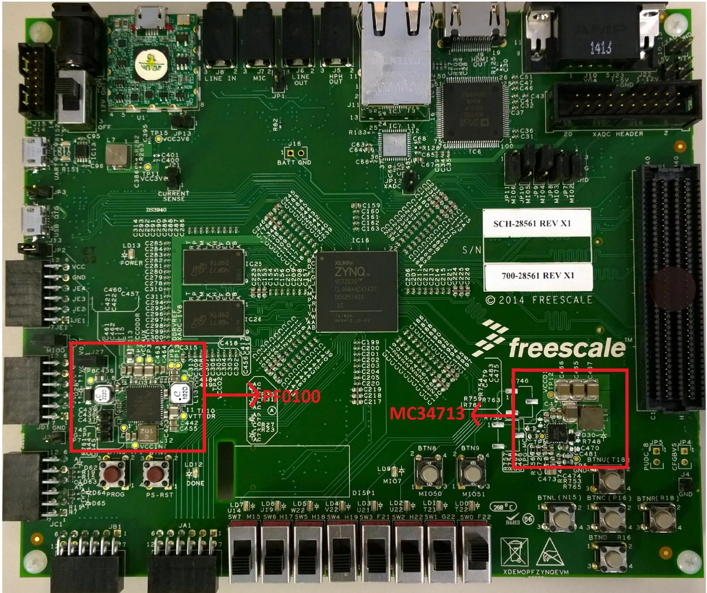
Figure 13. Zynq@-7020 board powered by PF0100
