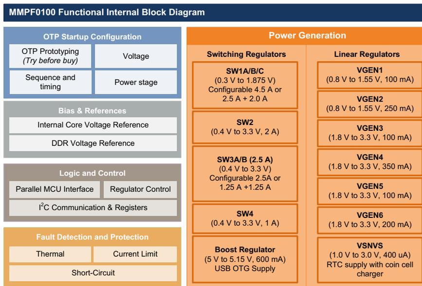
**Figure 3. Functional internal block diagram of the MMPF0100**
