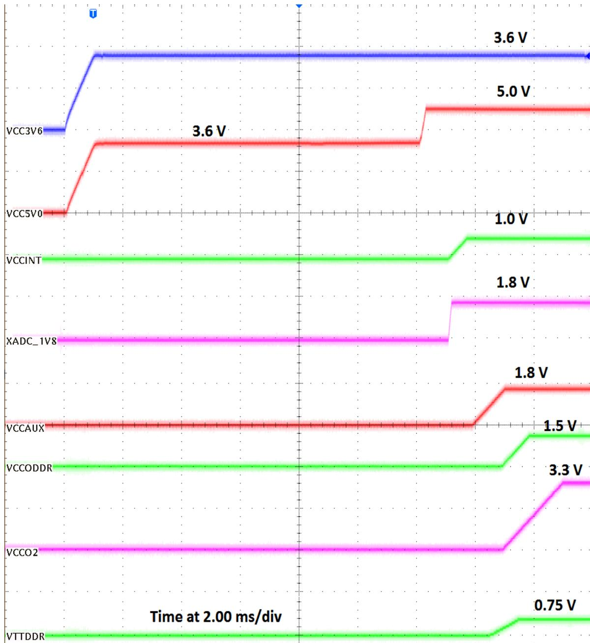
Figure 10. Power rails generated using the PF0100
