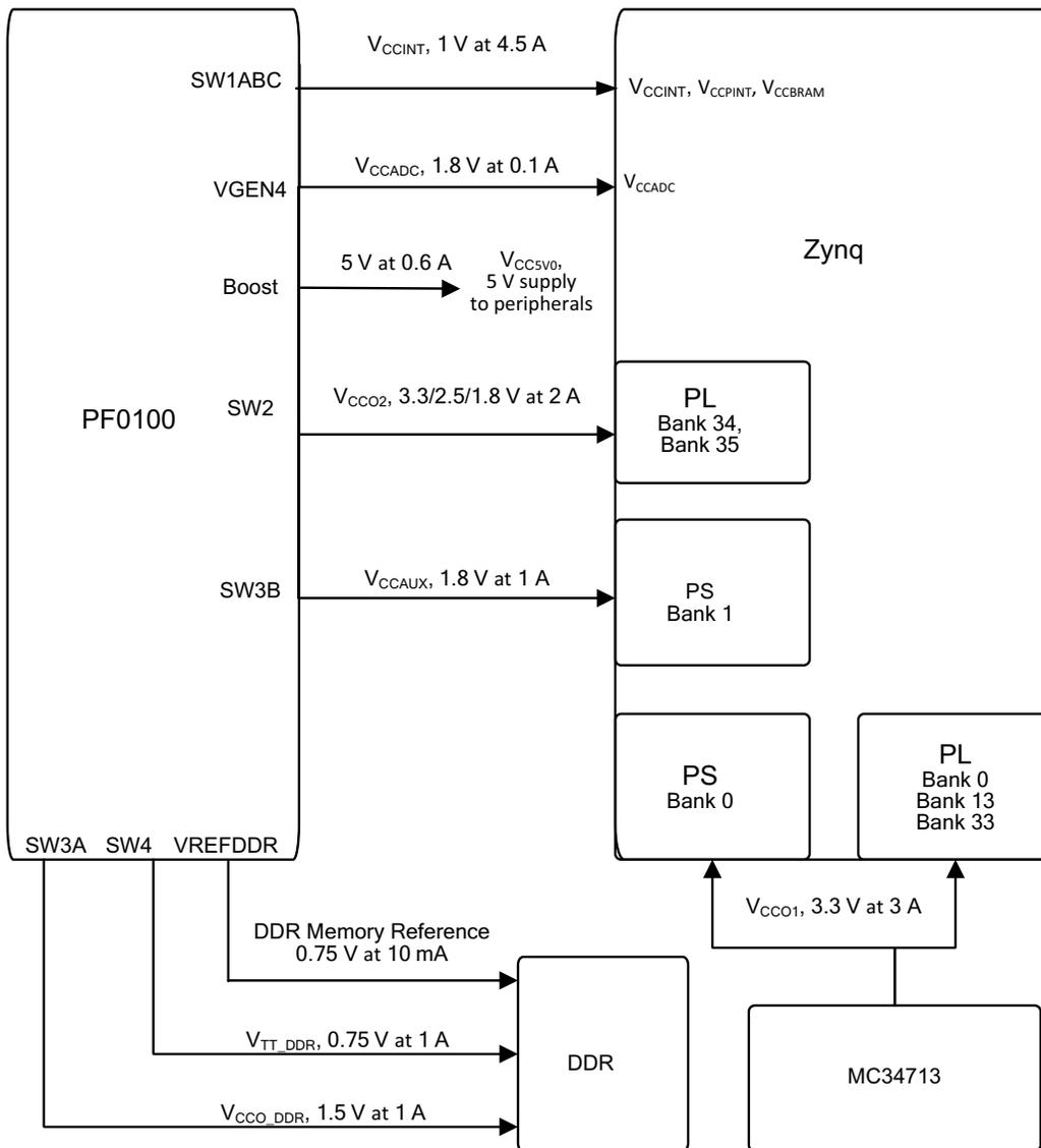
**Figure 9. Zynq® power bank assignments**
