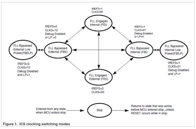
For this application note, the ICS is configured to FEI operation mode. The bus is configured to 20 MHz using an internal reference oscillator.
