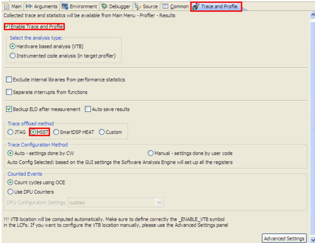
In **Advance Settings**, the path of the HSST data files needs to be specified for debug configurations associated with the cores.
