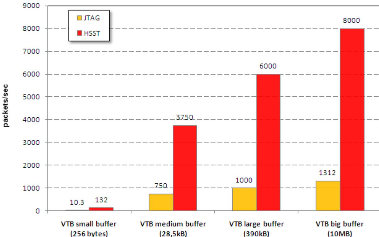
For large and big chunks of download data, the HSST is about six times faster than JTAG method.
