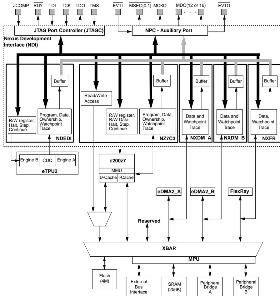
Figure 2. Typical MPC5600 Nexus Development Interface (MPC567xF shown)
