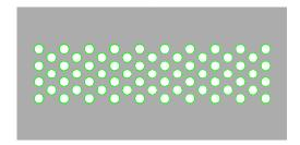
Figure 1c. Closeup of the PCB Via Layout with 12 mil Diameter Centers, 15 x 30 mil Pitch
