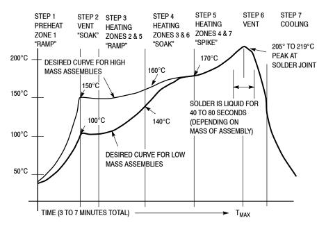
Figure 2. Typical Solder Heating Profile
