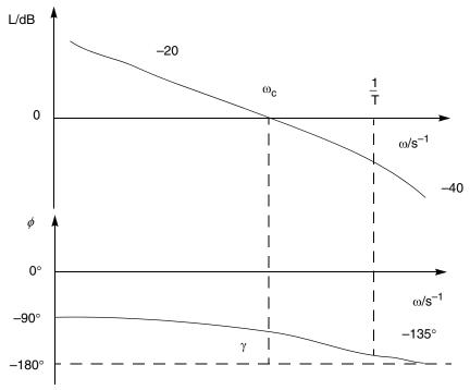
Figure 3. Bode Diagram of Type I System
