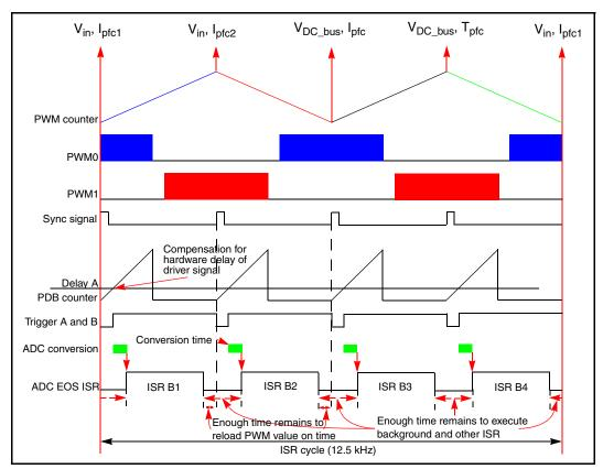
Figure 12. ADC Interrupt Control Sequence Diagram
