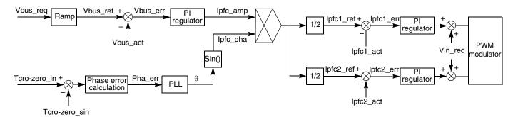
Figure 6. System Control Scheme of Single-Phase Two-Channel Interleaved Boost PFC Converter
