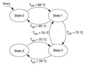
Figure 15. State Machine for Fan Speed Regulation
