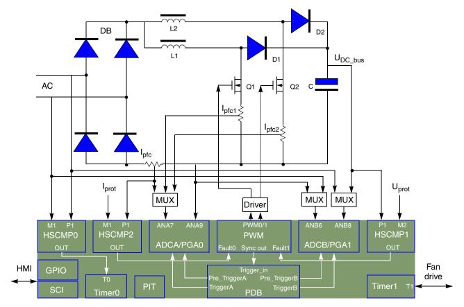
Figure 5. System Block Diagram for Single-Phase Two-Channel Interleaved Boost PFC
