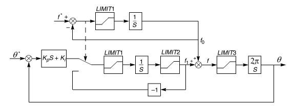
Figure 14. Input Voltage PLL Control Block Diagram
