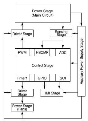
Figure 7. System Hardware Structure Block Diagram
