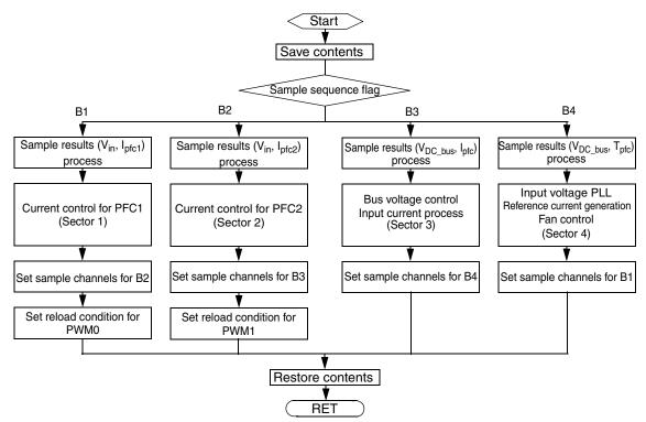
Figure 13. ADC ISR Flowchart
