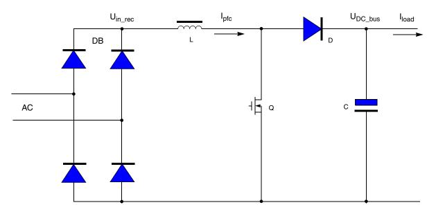
Figure 1. Single-Phase Boost PFC Converter Topology
