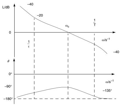
Figure 4. Bode Diagram of Type II System
