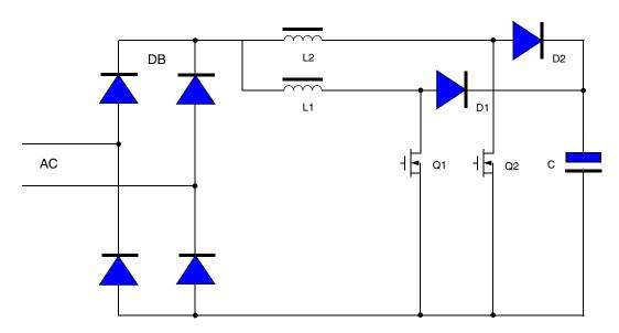
Figure 8. Main Power Topology Circuit
