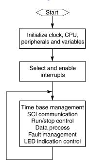
Figure 11. Main Loop Flowchart
