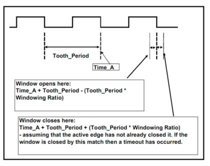
Figure 5. Mecanism for Windowing Out Noise
