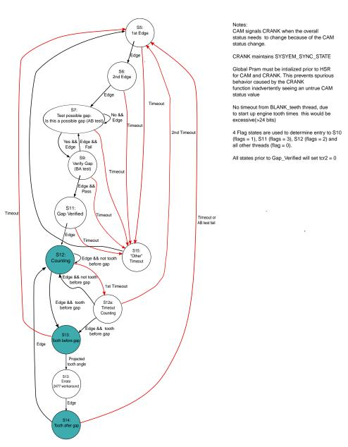
Figure A-2. Crank State Transition Part 2
