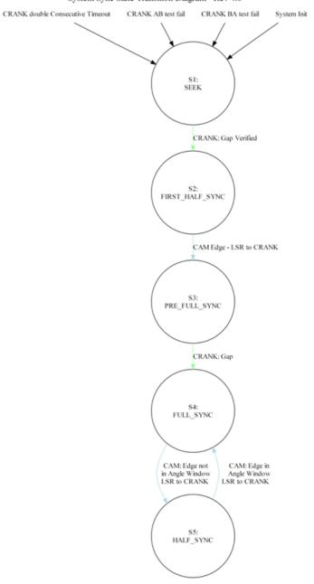
Figure C-1. System Sync State Transition
