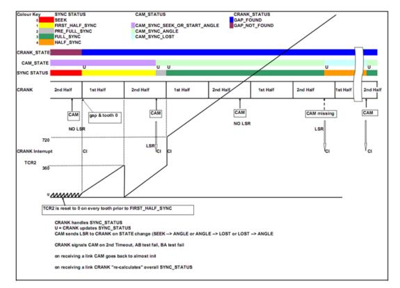
In this scenario, the cam edge occurs before the gap has been identified.
