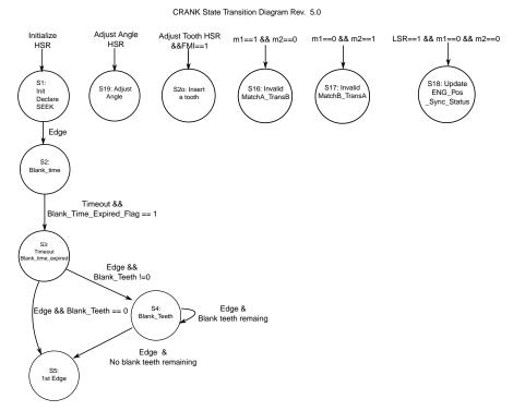
Figure A-1. Crank State Transition Part 1
