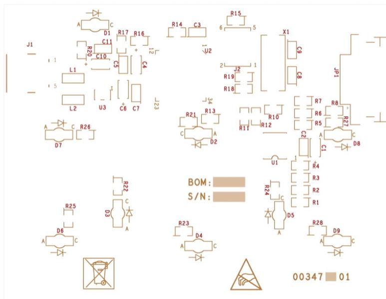
Figure 17. Bottom Component Placement on Demo Board (Not to Scale)
