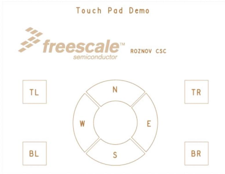
Figure 16. Pad Placement on Top Side of Demo Board (Not to Scale)
