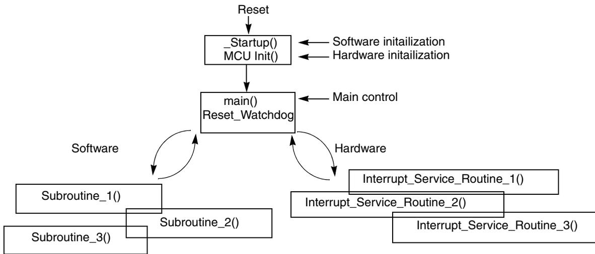
**Figure 2. Blood Pressure Monitor Software Flow**
