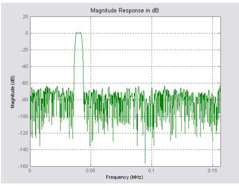
Figure 3. Frequency Response of the Quantized Bandpass Filter
