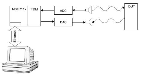
Figure 7. Layout for the Example Application
