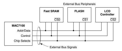
Figure 1-1. External Bus Structure
