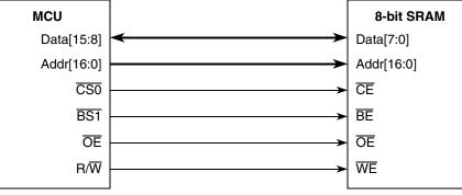
Figure 3-1. 8-bit External SRAM Example
