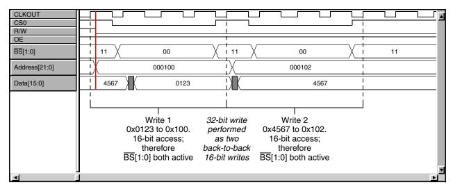
Figure 5-7. Test Case 6 (32-bit Write to 16-bit Port with 1 Wait State)
