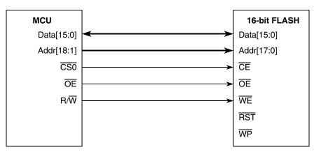
Figure 3-4. 16-bit External FLASH Example
