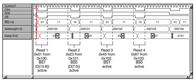
Figure 5-4. Test Case 3 (4 x 8-bit Reads with 1 Wait State)
