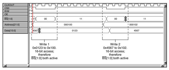
Figure 5-5. Test Case 4 (2 x 16-bit Writes with 1 Wait State)
