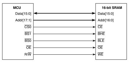
Figure 3-3. 16-Bit External SRAM Example
