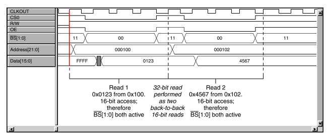
Figure 5-8. Test Case 7 (32-bit Read to 16-bit Port with 1 Wait State)
