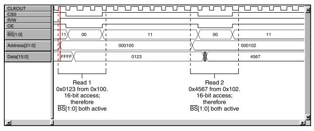
Figure 5-6. Test Case 5 (2 x 16-bit Reads with 1 Wait State)
