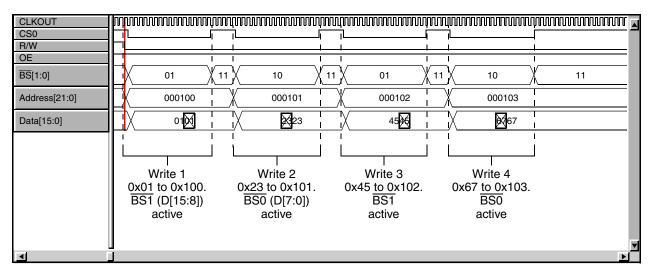
Figure 5-3. Test Case 2 (4 x 8-bit Write With Default CS0 Configuration, Maximum Wait States)
