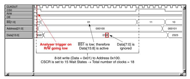
Figure 5-2. Test Case 1 (8-bit Write to 0x100 With Default CS0 Configuration, Maximum Wait States)
