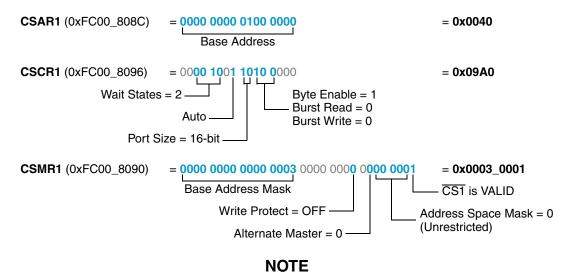
The memory range defined for chip select  $\overline{\text{CS1}}$  does not overlap the previous chip select  $\overline{\text{CS0}}$  memory range. This is a requirement of the configuration. Overlapping memory ranges must be avoided or unpredictable results will occur.
